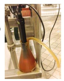
Whether measuring in bright beer or wort, it is imperative that all gases are in solution before oxygen is measured by the analyzer. Soluble gases such as oxygen are displaced by bubbles, which artificially reduce the dissolved concentration value.
