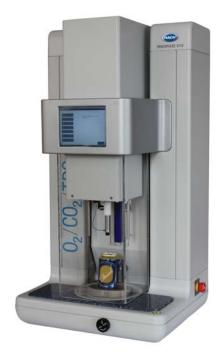
c) Always shake packages vigorously before piercing to equilibrate the head space and dissolved gases. TPO concentrations are based on shaken package measurements.
