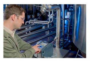
Be aware that the first measurement of the day will have a slower response, since the sensor must rid itself of any air accumulated in the instrument. It must also adjust to the beer temperature.
